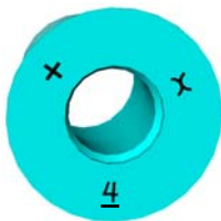
Illustration of head markings on HR3252-5-04
