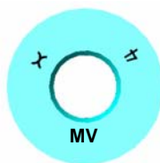
Illustration of head markings on UB100-MV06-04
