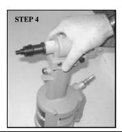
STEP 4 Attach sleeve adapter to tool housing and tighten with wrenches
