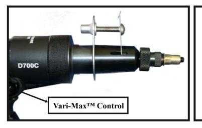
The **D-700-VM Vari-Max<sup>™</sup>** feature enables the user to set a pull force when upsetting a blind rivet nutor insert to help insure a proper installation without damaging the threads of the blind nut insert or the threads on the pull-up stud. The normal operating range for the D-700-VM is 1000 to 5,000 lbs. The Vari-Max<sup>™</sup> is located on the tool on the side opposite the release button (right side of the tool facing forward).
