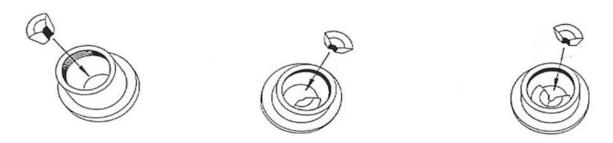
4. When the jaws are in place, insert **Jaw Holder** into **Spring**, being sure to keep large end of **Jaw Holder** pointing downward.
